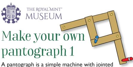
A pantograph is a simple machine with jointed arms that can copy or draw pictures at different sizes. Before the invention of computers, The Royal Mint used special machines that work in the same way as a pantograph in its coin-making process. These were called reducing machines and they were used to trace large coin designs and scale them down to life-size coin copies. Try making your own cardboard pantograph and then experiment with enlarging and reducing pictures.
