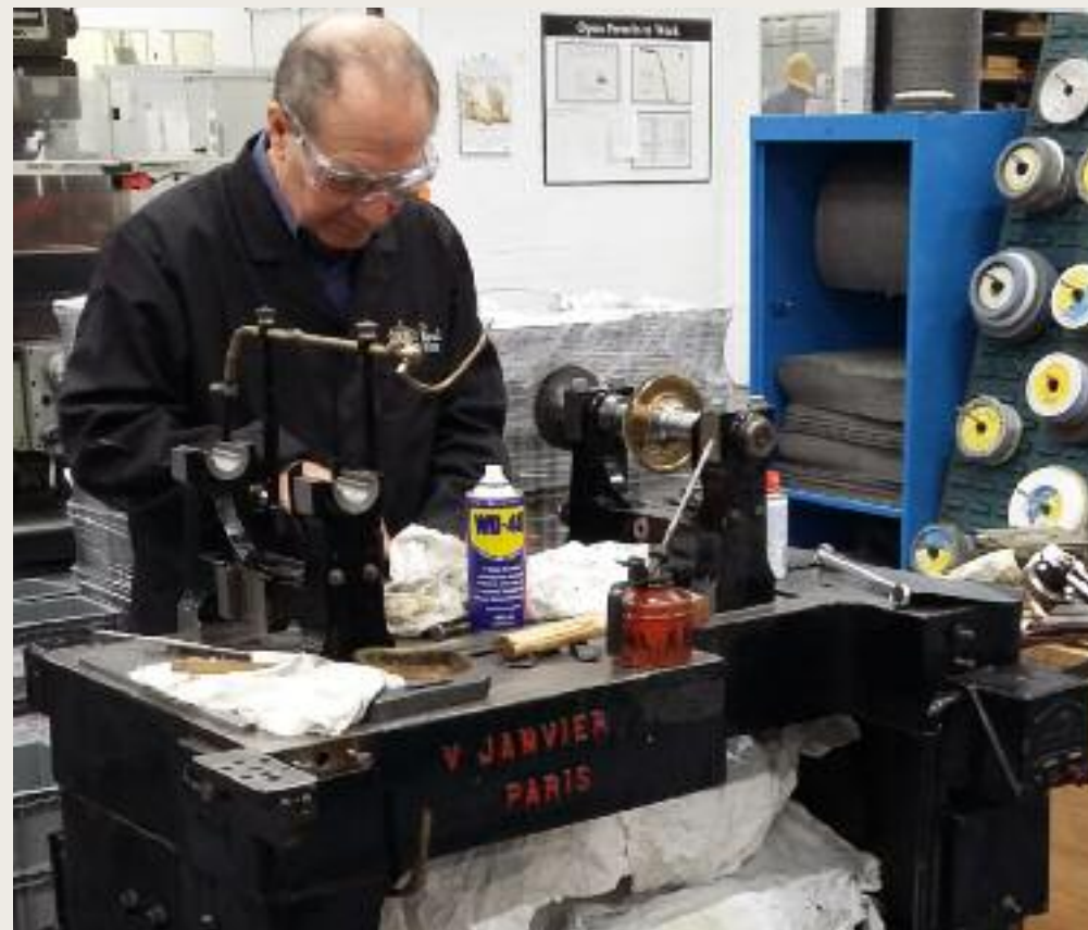
Above: Ken Stoa restoring the Janvier reducing machine. Ken had been responsible for the operation and maintenance of all the reducing machines at The Royal Mint before his retirement.
